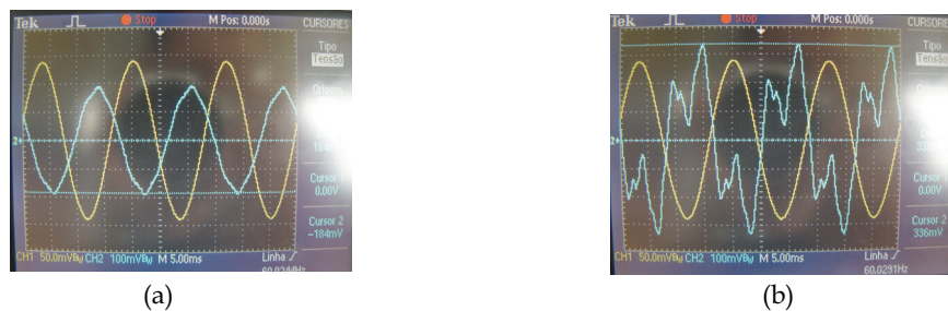
Fig. 10. Waveforms of the leakage current (blue) and of the applied voltage (yellow), (a) CT in the position 1 and (b) CT in the position 2.
