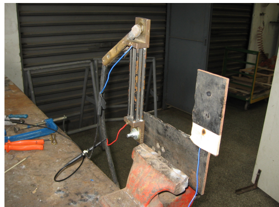
Figure 3: Resistor shunt used for current measurement.
