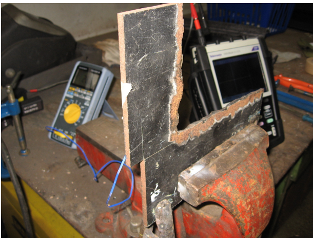
Figure 6: Sheet steel used in the tests caught in the vise.
